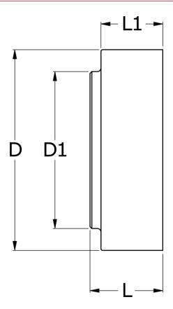
D = 480 D1 = 300 L = 190 L1 = 90 Max bore = 180 Torque (N m) = 16600
